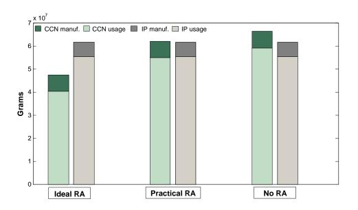
Figure 1: Carbon footprint for CCN and IP-based networks
