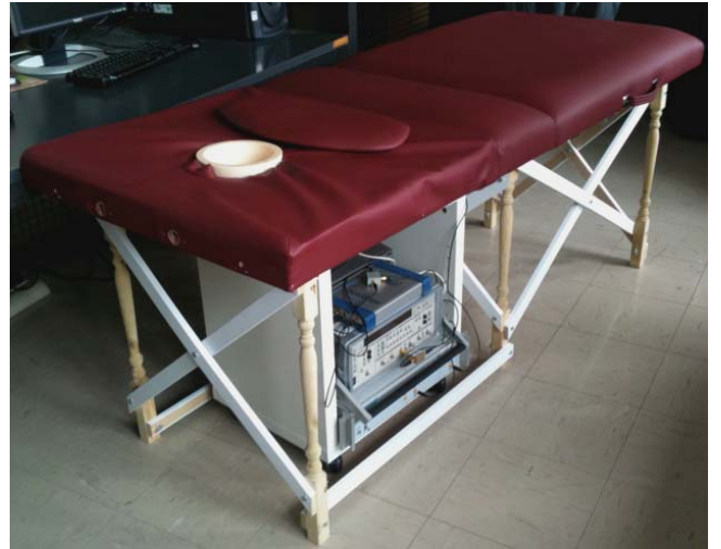
Fig. 1. Photograph of the breast imaging measurement system and its patient interface.
