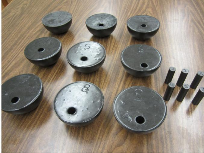
Figure 2: The breast phantoms and plugs constructed to collect the phantom measurements in controlled experiments.
