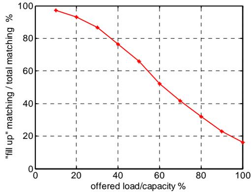
Figure 3.6: ratio of “fill up” matching over total number of matching vs. offered load
