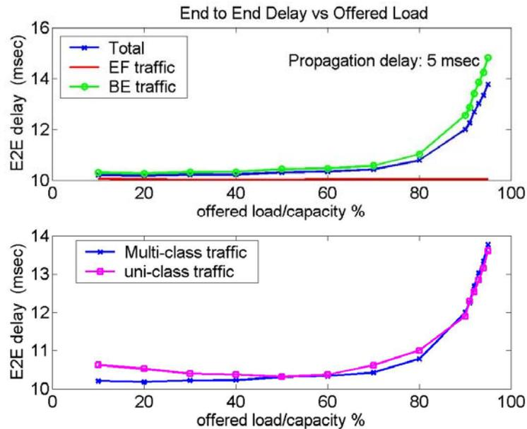
Figure 5.10: Differentiated service performance: End to end delay vs. offered load
