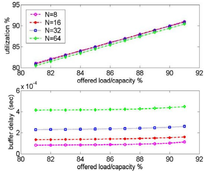
Figure 5.7: Adapted PIM performance with network size scaling up ( $N$  is the number of edge nodes in AAPN): top panel: Utilization vs. offered load; bottom panel: average buffer delay vs. offered load
