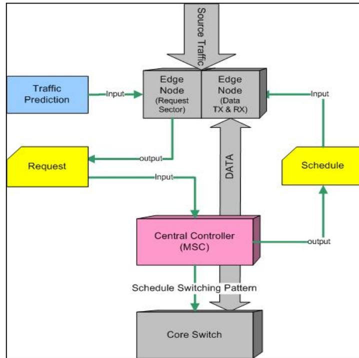
Figure 4.5: Frame based scheduling system for Frame
