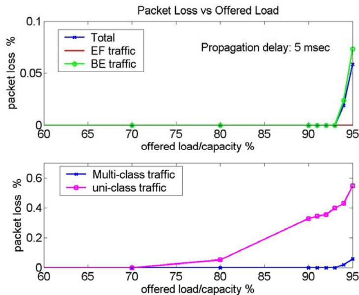
Figure 5.9: Differentiated service performance: Packet loss vs. offered load
