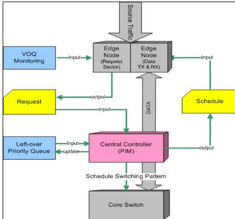
Figure 4.3: Logic diagram for slot based scheduling system
