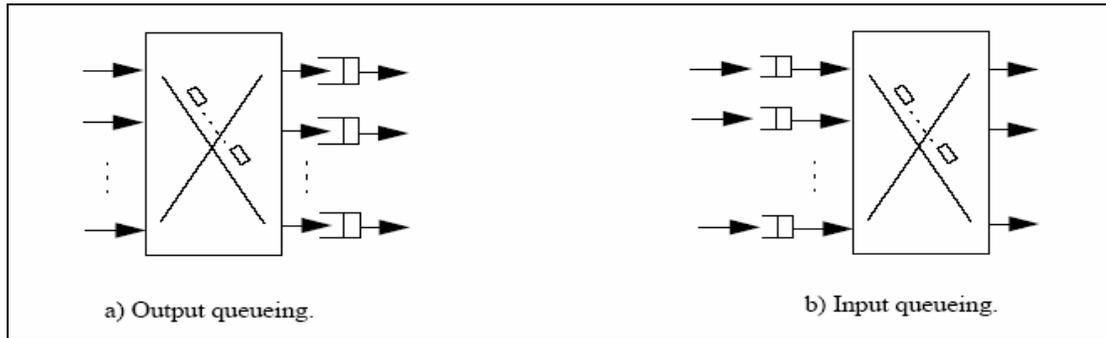
Figure 3.2: Output queuing and Input queuing
