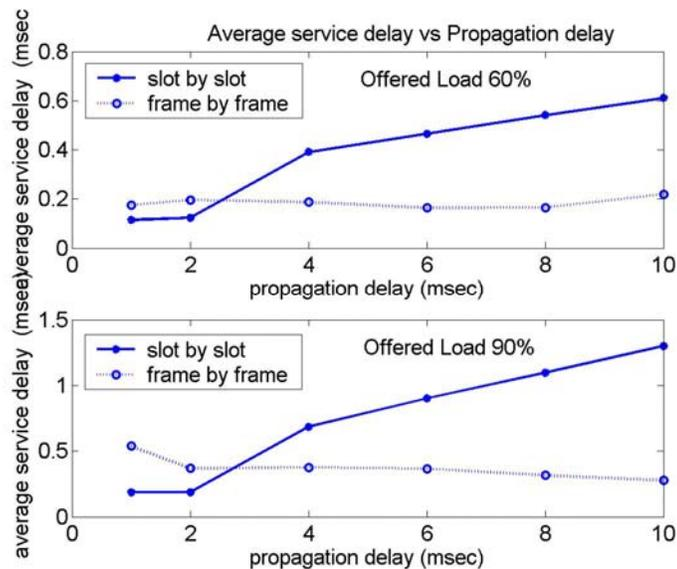
Figure 5.11: Average service delay as a function of propagation delay in uniform traffic scenario. Top panel: Offered load of 60%. Bottom panel: Offered load of 90%.
