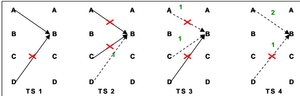
Figure 3.5: Example of weighted matching for one output over 4 time-slots
